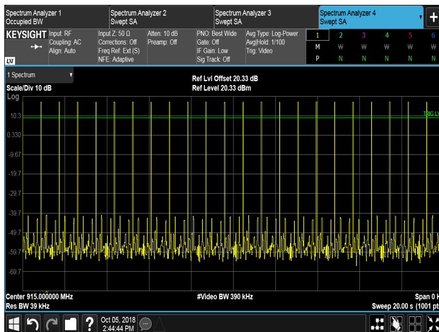
Figure 7 - 915 SRD frequency-hop packet, Total Average Time of Occupancy
