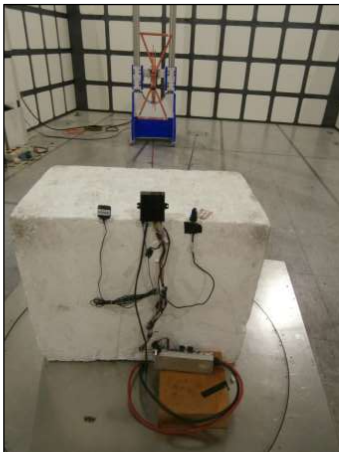
Figure 63 - Test Setup - 30 MHz to 1 GHz – Y Orientation
