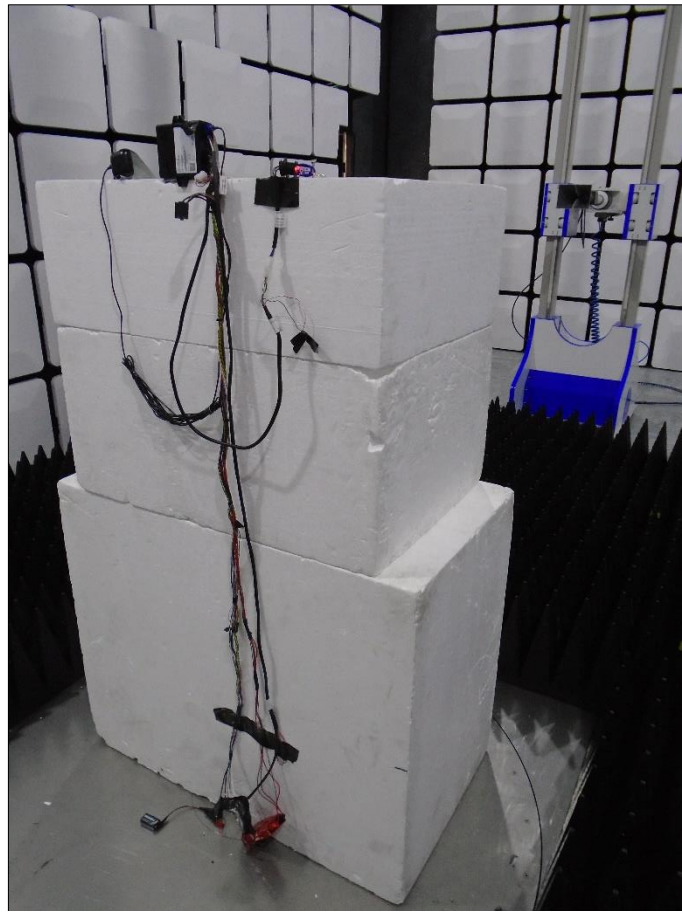
Figure 50 - Test Setup - 1 GHz to 18 GHz - Z Orientation
