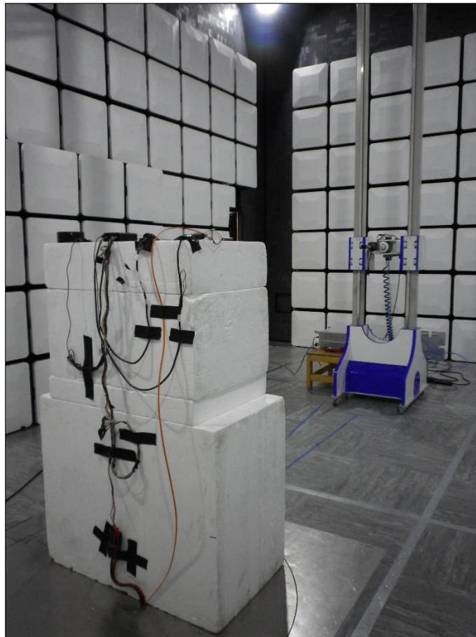
Figure 51 - Test Setup - 18 GHz to 25 GHz - X Orientation
