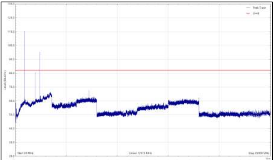
Figure 14 - 2441 MHz, 915 MHz and 1880 MHz, 30 MHz to 25 GHz, Orientation X, Vertical (Peak)
