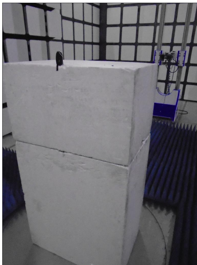
Figure 70 - Test Setup - 1 GHz to 18 GHz - Y Orientation
