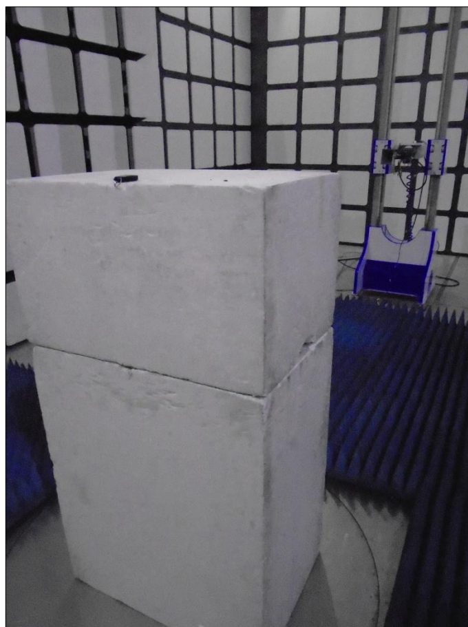
Figure 69 - Test Setup - 1 GHz to 18 GHz - X Orientation
