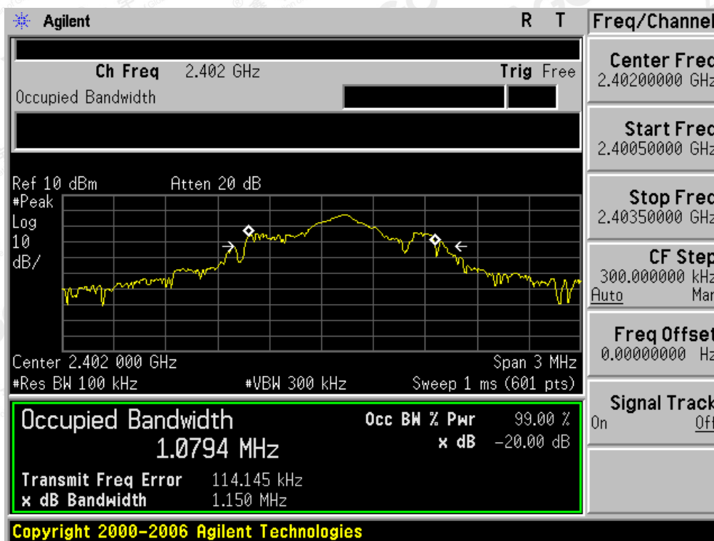
TEST PLOT OF BANDWIDTH FOR LOW CHANNEL
