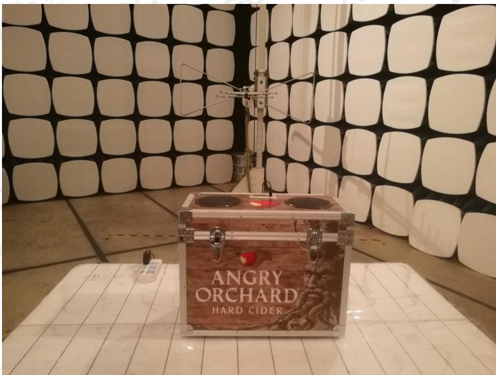
FCC RADIATED EMISSION TEST SETUP
