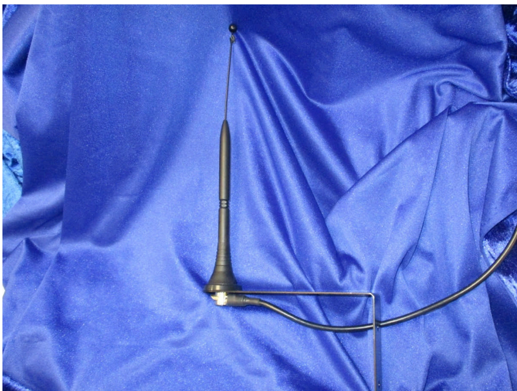
Photograph shows the 915MHz UHF antenna
