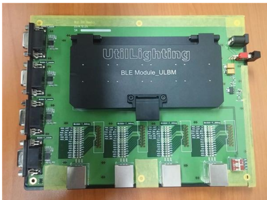
Figure 5-1 Zig Board for Mass Production (1)
