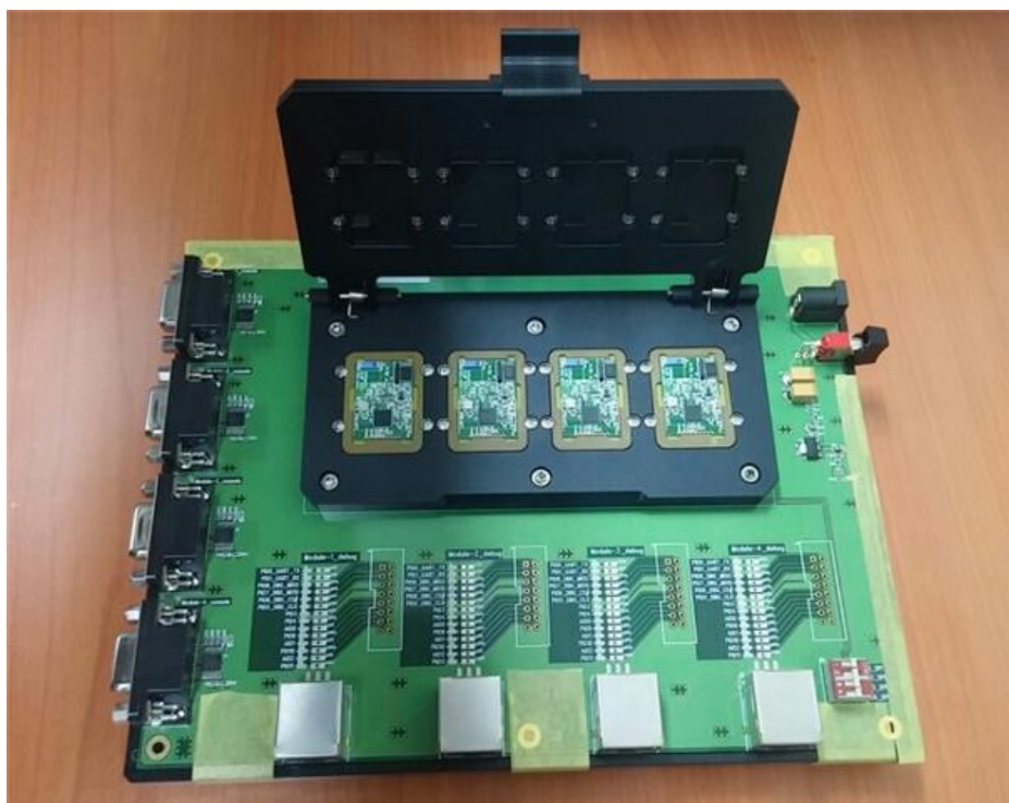
Figure 5-2 Zig Board for Mass Production (2)
