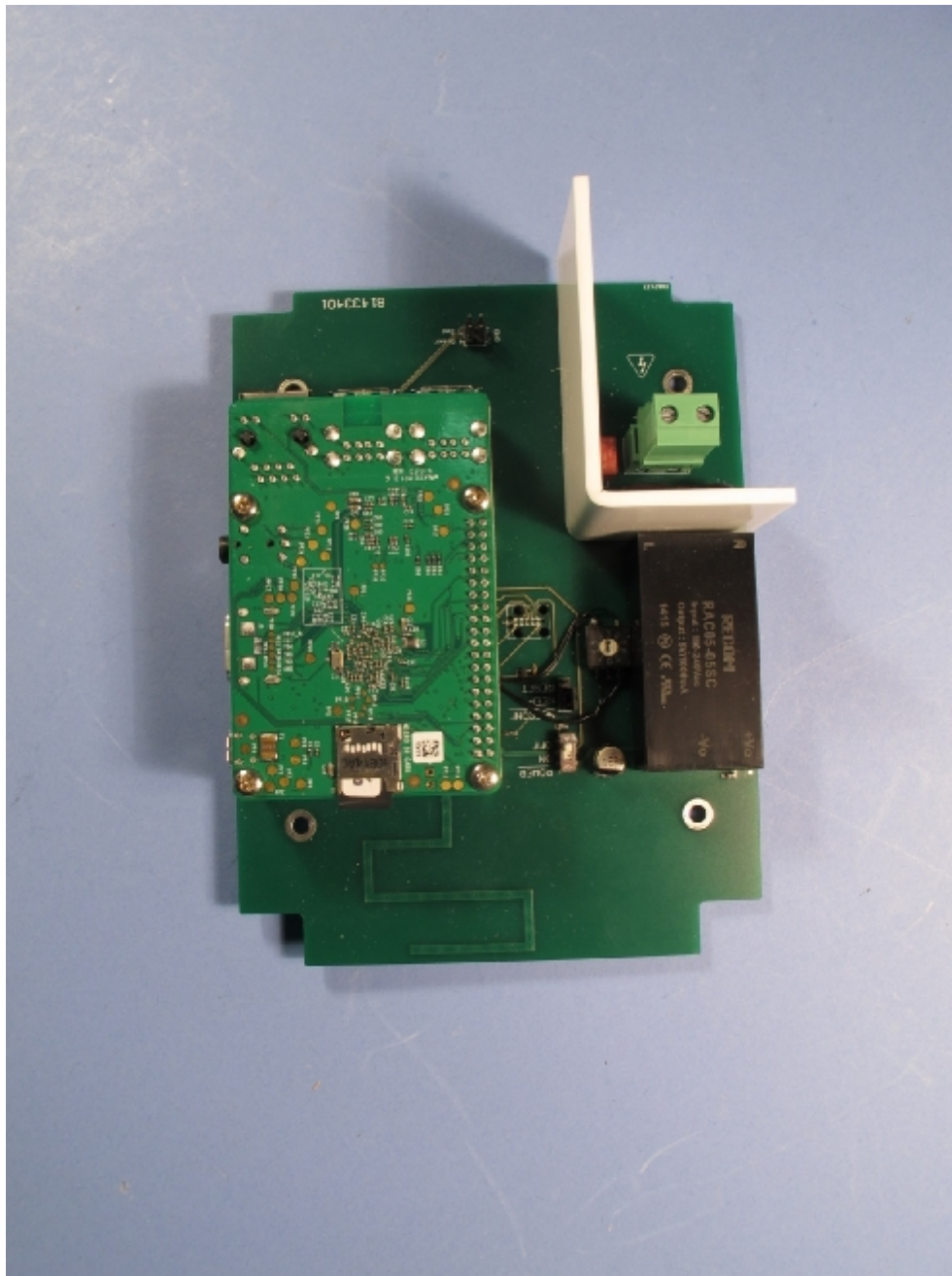
Photograph 2: PCB top view of Concentrator
