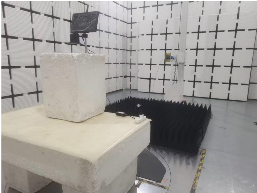
Set-up for Radiated Spurious Emission, Above 1GHz
