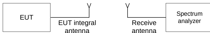
Figure 7.1.1 Setup for transmitter shut down test
