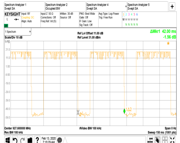
Plot 7.5.4 Pulse duration and pulse period test result
