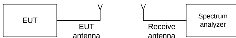
Figure 7.3.1 Occupied bandwidth test setup
