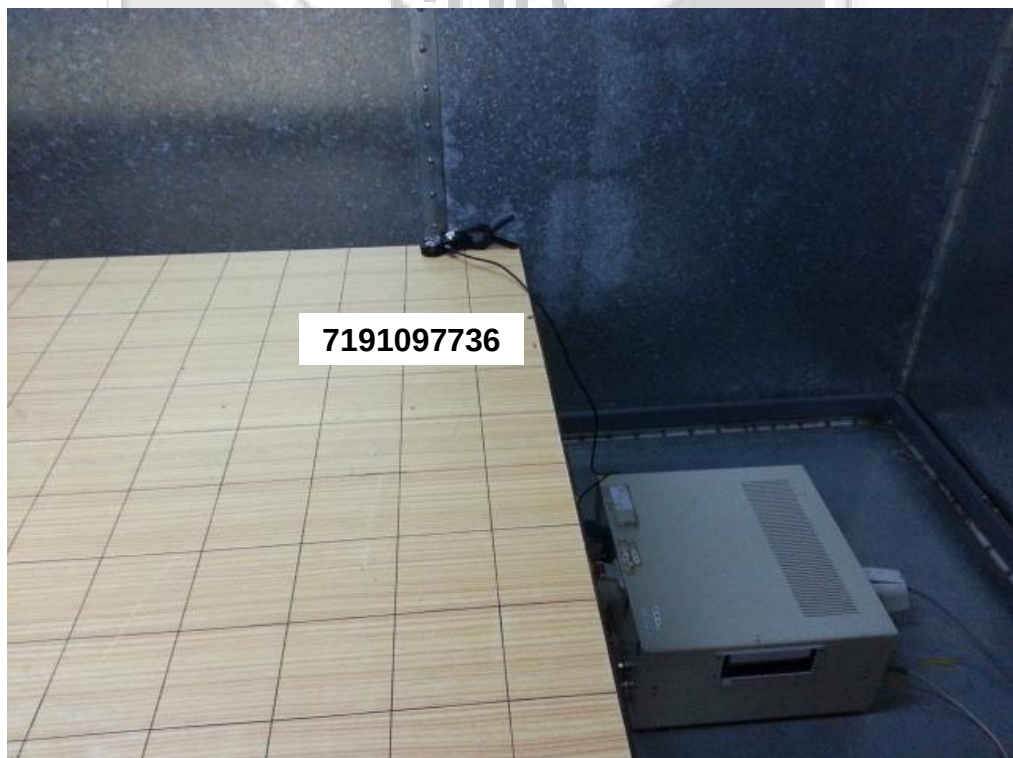
Conducted Emissions Test Setup (Rear View)
