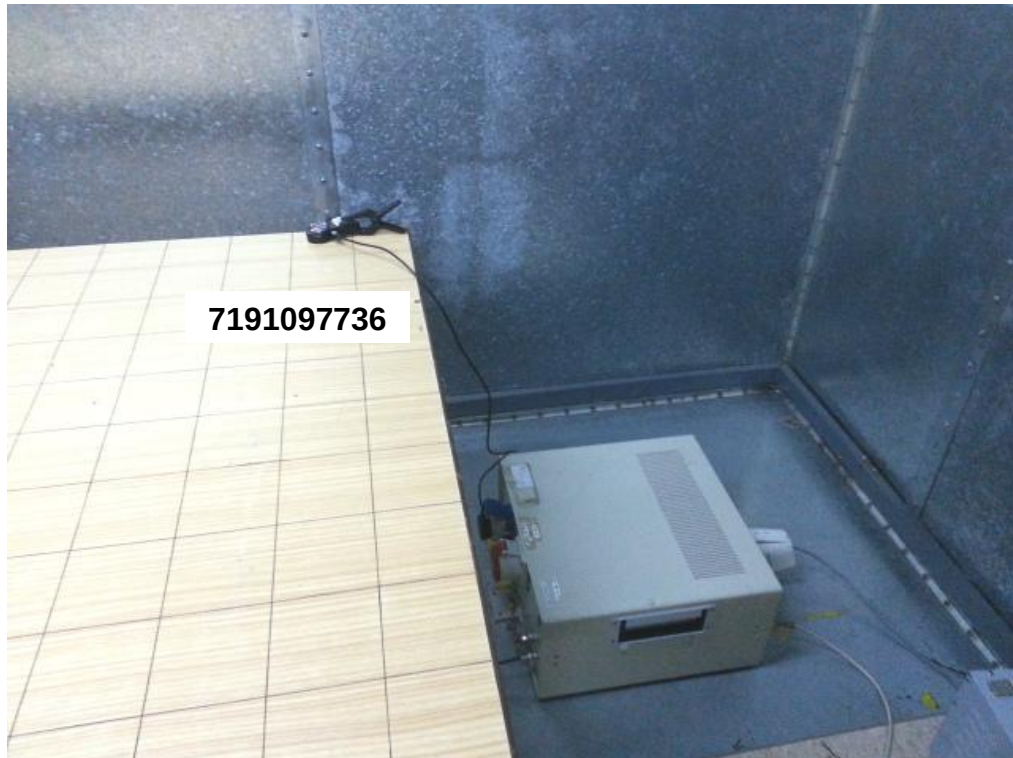
Conducted Emissions Test Setup (Front View)
