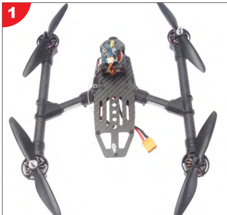
1 Installed the four rotors in properly.
