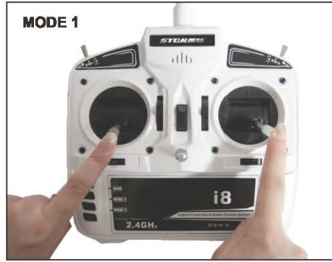
Mode1 Radio, compass calibration process: Put the Elevator stick to the bottom position, and push the Throttle stick to the end corner of right .
