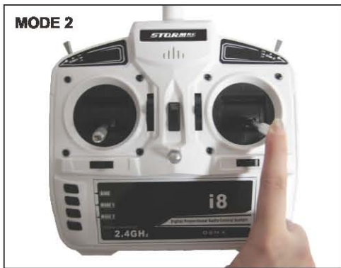
Mode2 Radio, compass calibration process: Put the throttle stick to the bottom position, and push the Aileron stick to the end corner of right .
