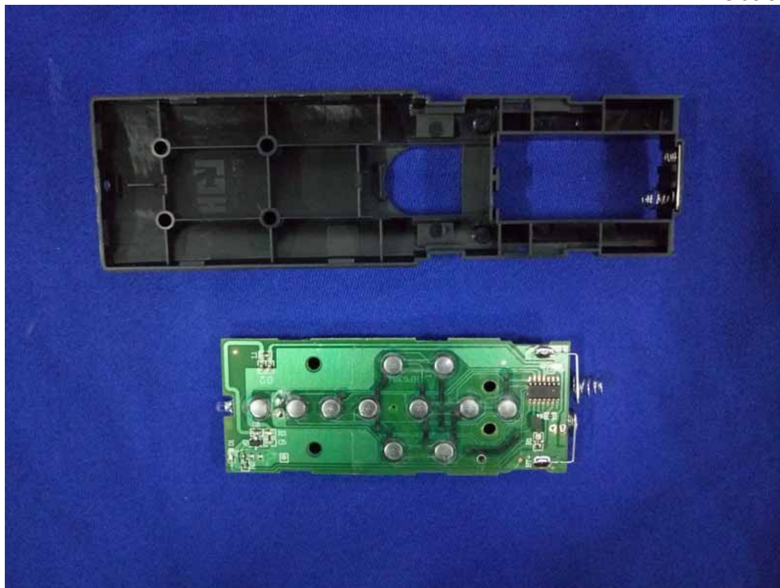
Figure 11 Inside of the EUT
