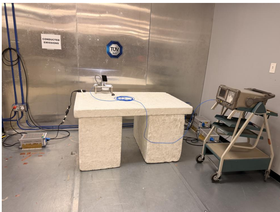
Figure 6: EUT – Power Line Conducted Emissions Test Setup
