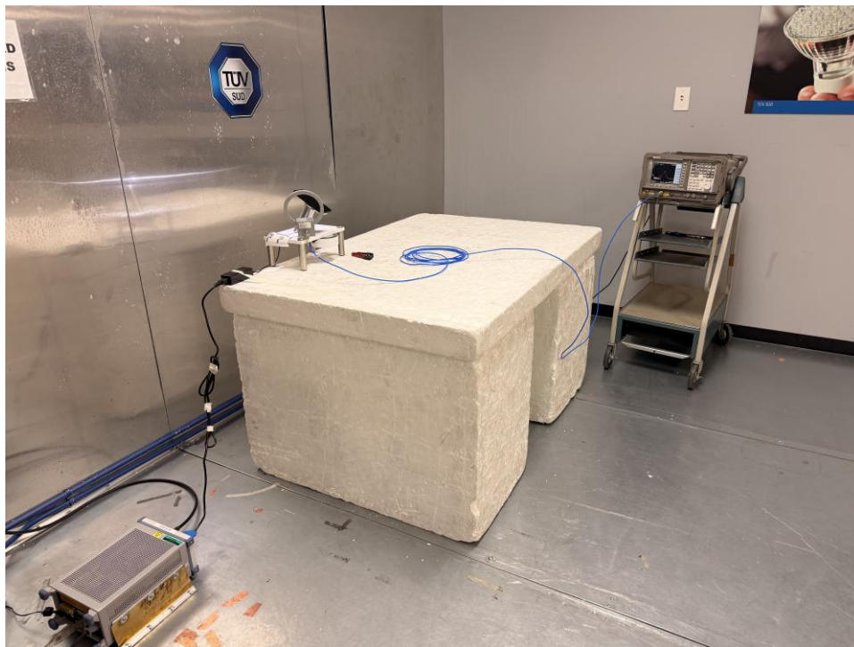
Figure 5: EUT – Power Line Conducted Emissions Test Setup
