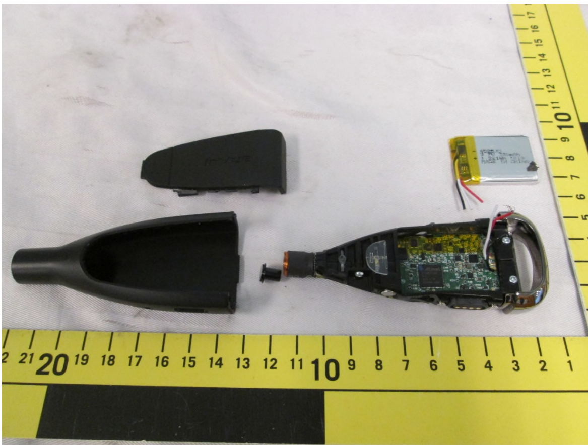
EUT – Internal view 1 Cover & battery removed
