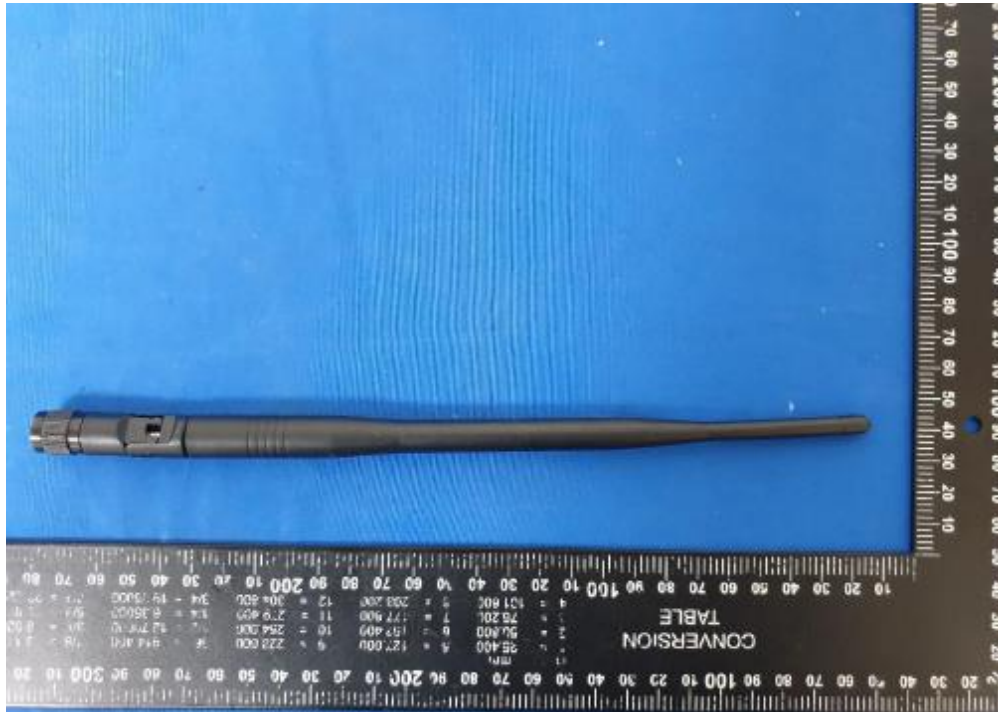
Dipole Antenna (TAOGKAS GW.71.5153)
