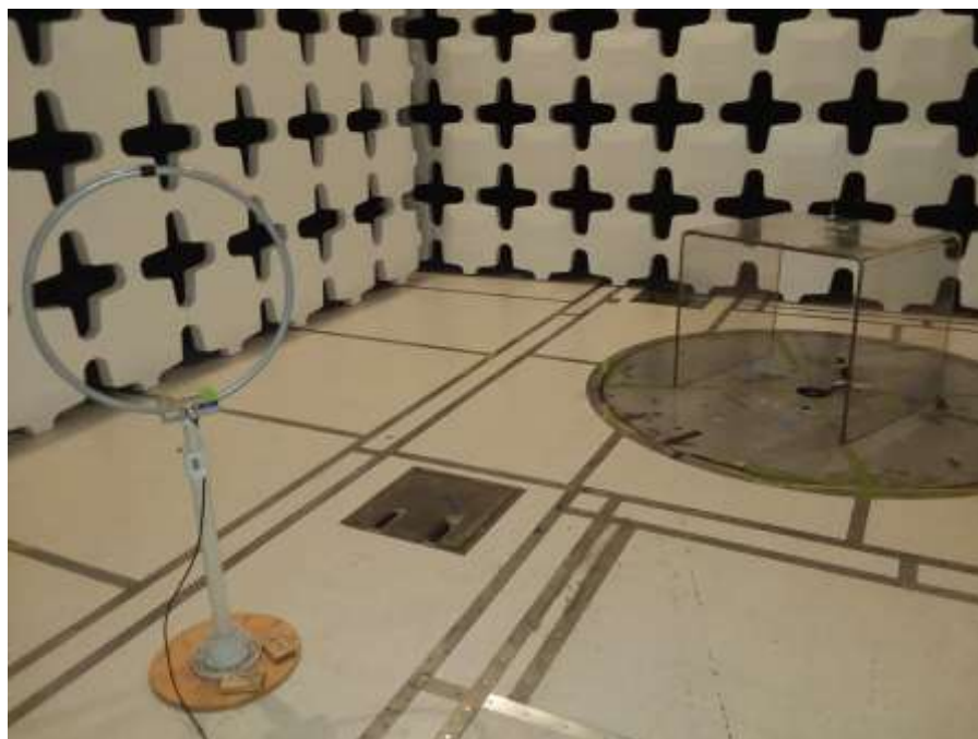
Figure 16. Radiated Emissions, Below 30 MHz, Perpendicular, Vertical Unit, Test Setup
