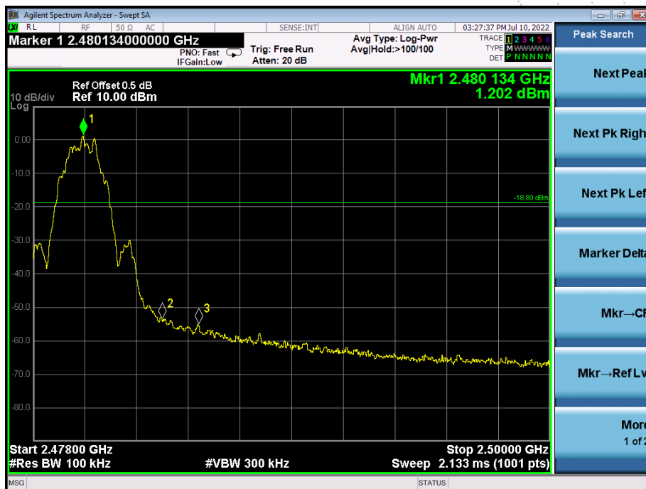
GFSK: Band Edge, Right Side
