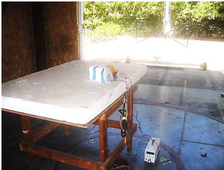
EKKO EK-1 Test Setup, 1 – 25GHz
