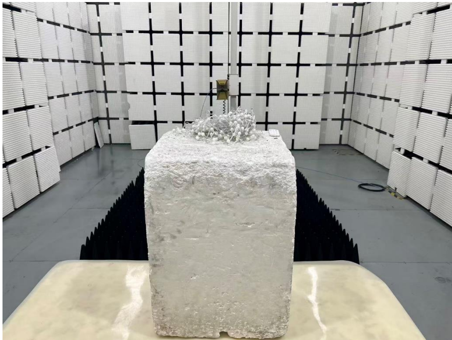
Set-up for Radiated Spurious Emission, Above 1GHz
