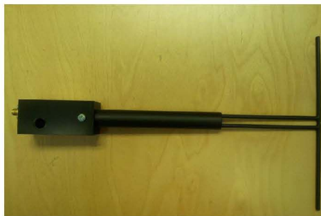
Figure 1 – MVG COMOSAR Validation Dipole
