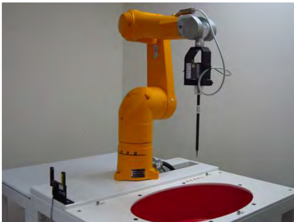
Fig.1 Photograph of the SAR measurement system
