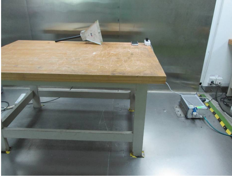
Conducted Emissions - Front View
