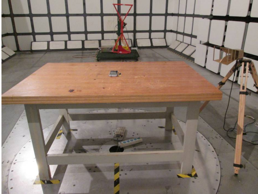
Radiated Emissions View (Below 1GHz)
