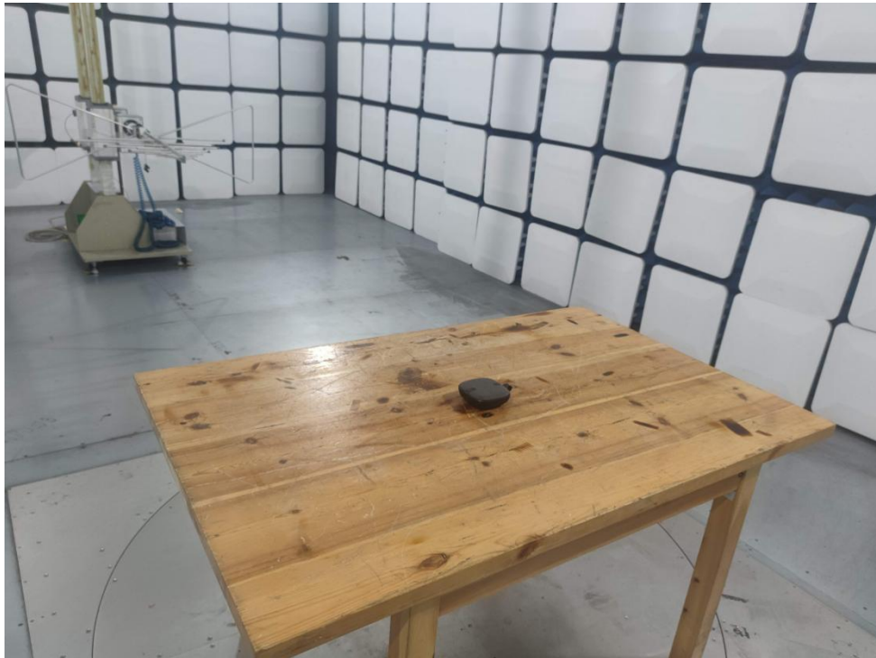
Photo of Radiation Emission Test
