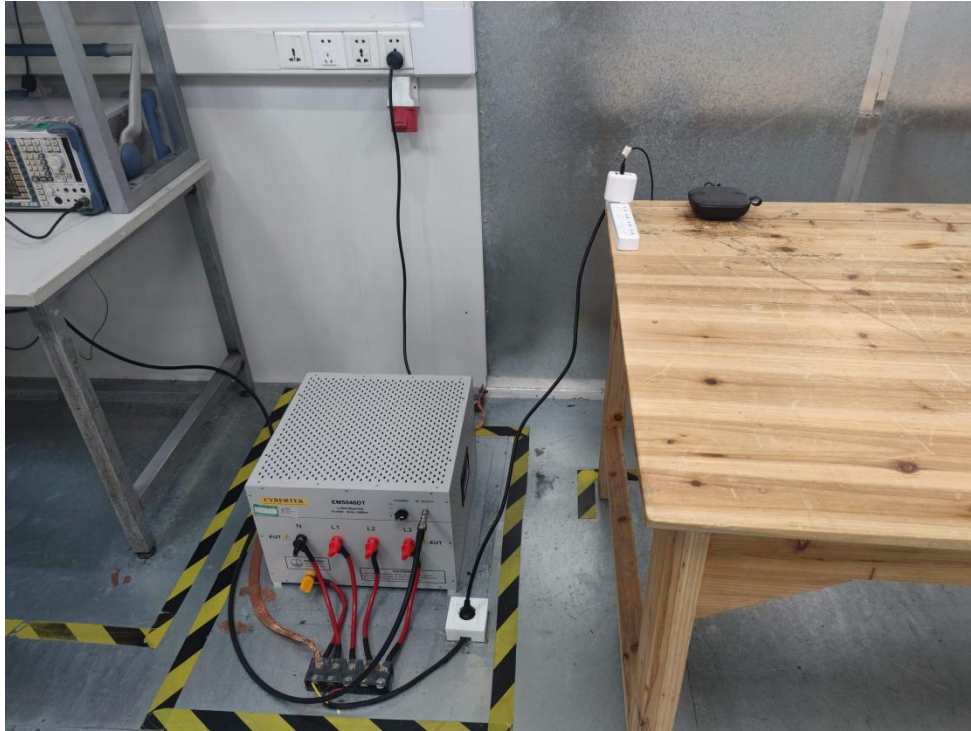
Photo of Conducted Emission Measurement
