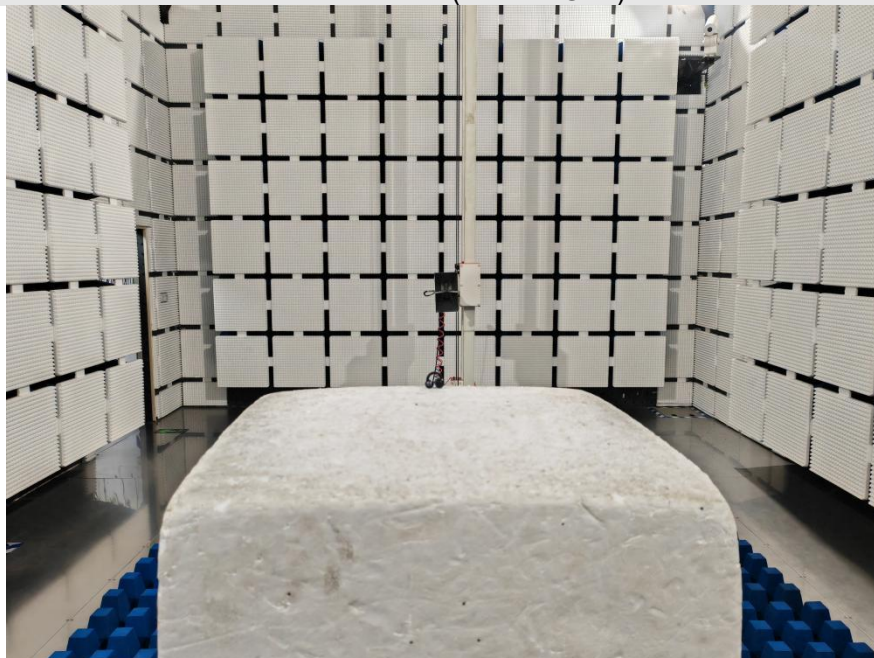
Radiated Emissions (above 1GHz) L ear
