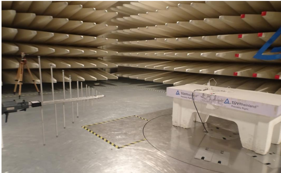
Photo 5: Log periodic antenna Vertical polarization with adapter 1
