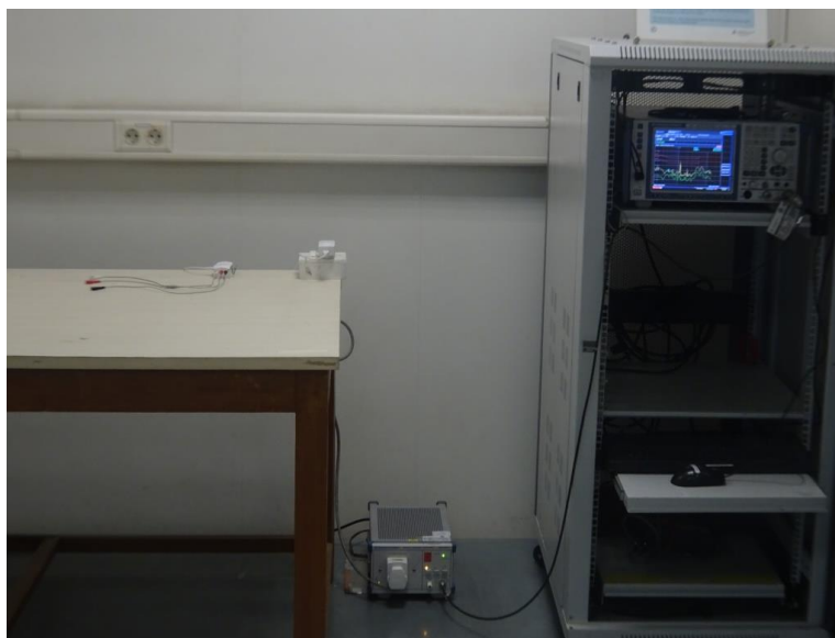
Photo 16: Conducted emission setup with adapter 2
