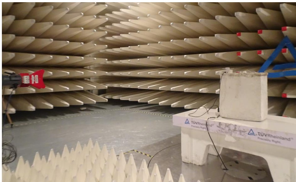
Photo 12: Horn antenna with horizontal polarization
