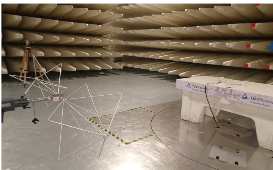
Photo 4: Biconical antenna Horizontal polarization with adapter 2
