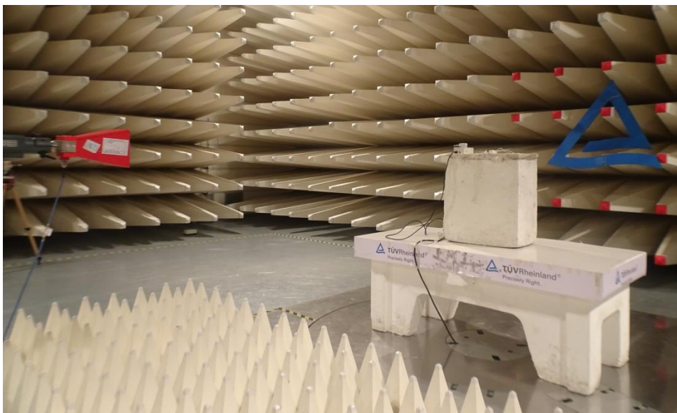
Photo 9: Horn antenna with vertical polarization
