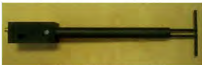
Figure 1 – MVG COMOSAR Validation Dipole
