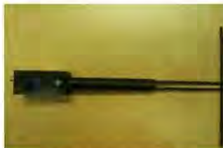
Figure 1 – MVG COMOSAR Validation Dipole
