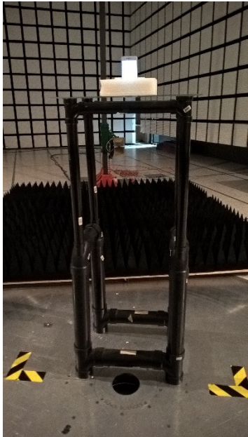
Figure 3.6-3: Setup photo – Radiated Emissions above 1GHz
