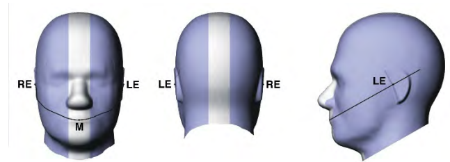
Figure 3.2 Front, back and side view of SAM
