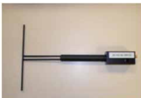
Figure 1 – Satimo COMOSAR Validation Dipole
