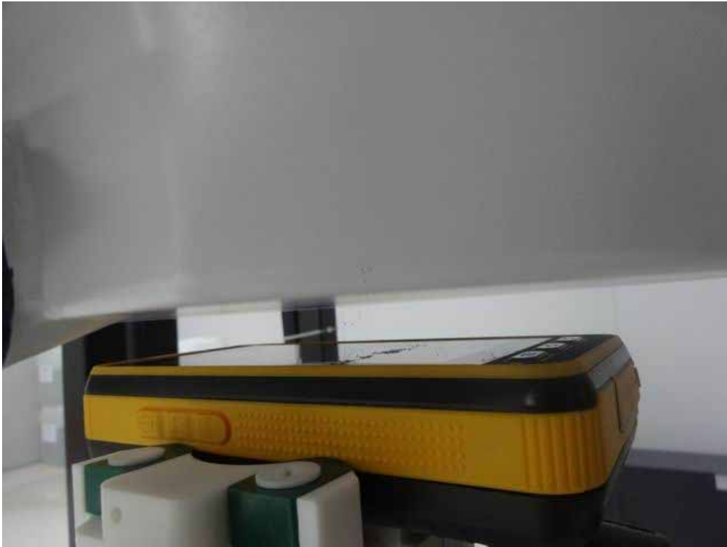
15mm body-worn Front Side Setup Photo
