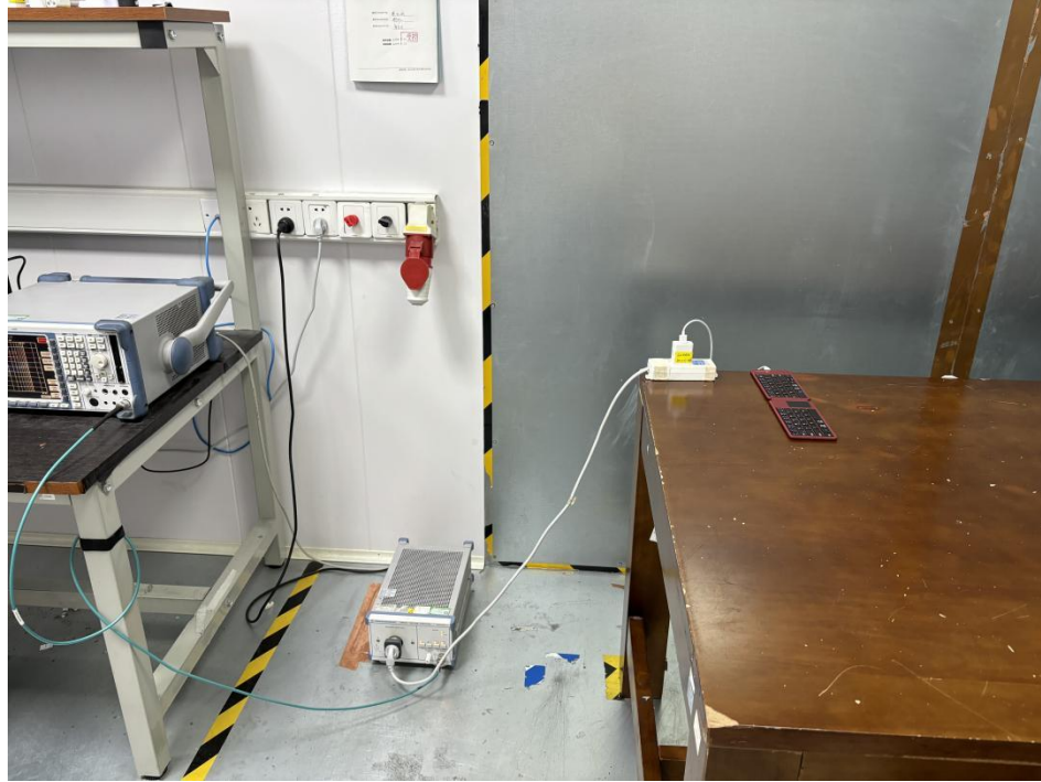
Conducted Emissions at Mains Terminals (150kHz-30MHz)
