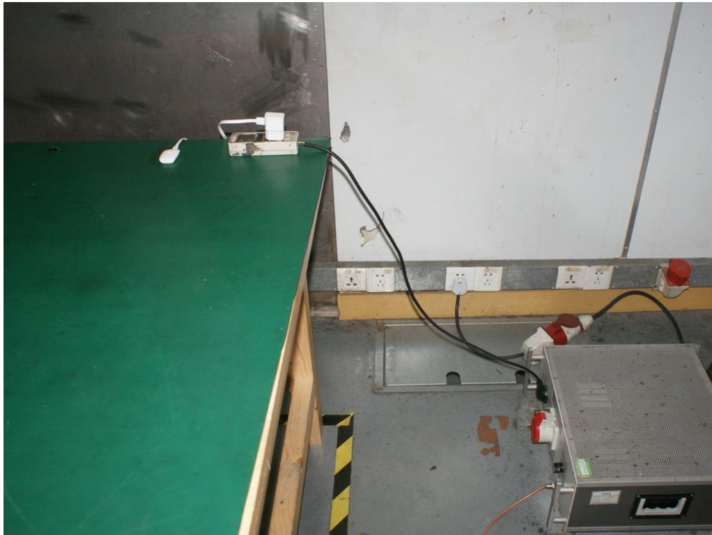
Photograph 3: Set-up for Conducted emissions, UpRight Battery Charging with AC/DC adapter
