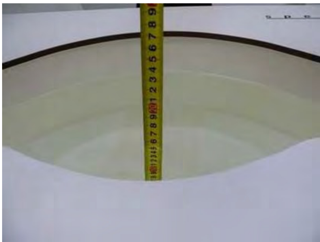
Picture 20: Liquid depth in the flat Phantom (5800 MHz, 15.0cm depth)
