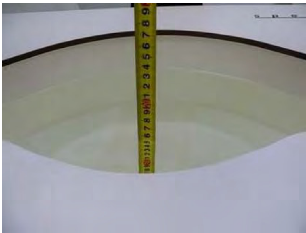
Picture 14: Liquid depth in the flat Phantom (2600 MHz, 15.3cm depth)
