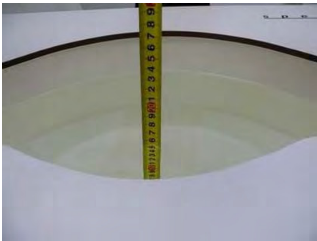
Picture 18: Liquid depth in the flat Phantom (5600 MHz, 15.3cm depth)
