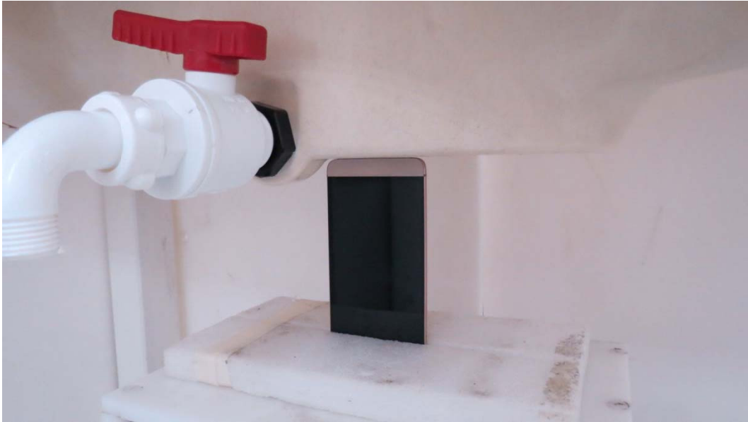
Picture 18: Bottom Side, the distance from handset to the bottom of the Phantom is 0mm
