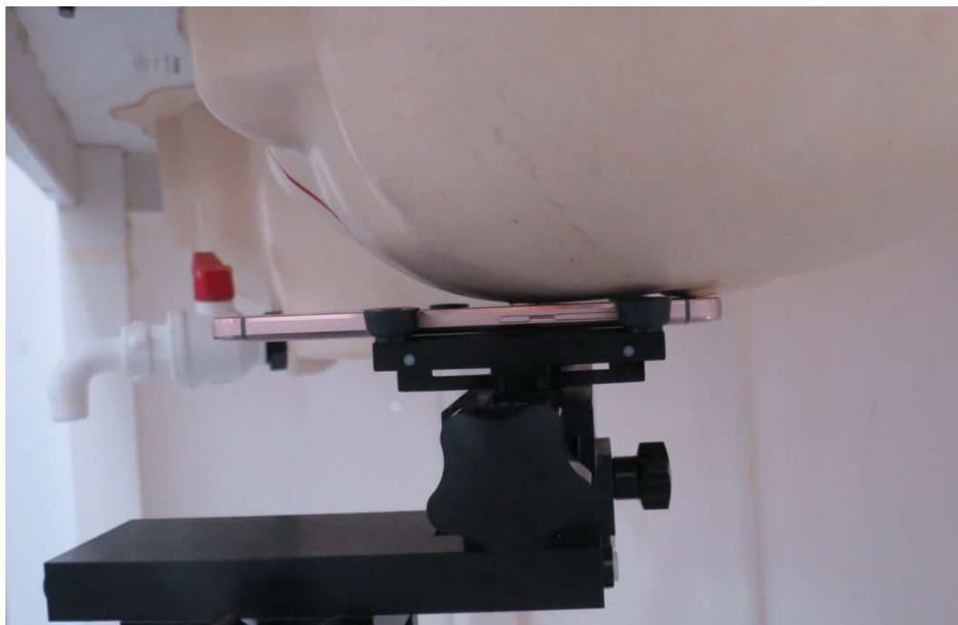
Picture 2: Left Hand Touch Cheek Position
