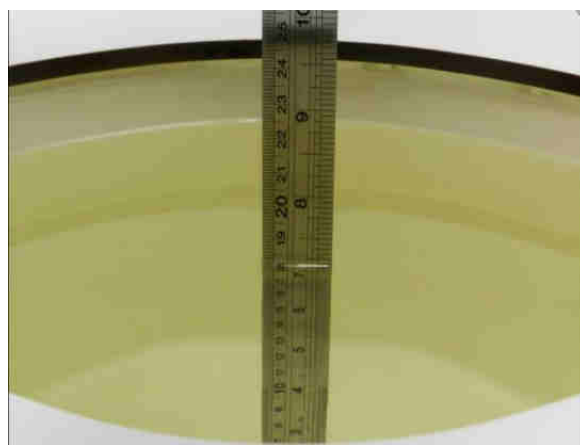
Fig 10.2 Photo of Liquid Height for Body SAR
