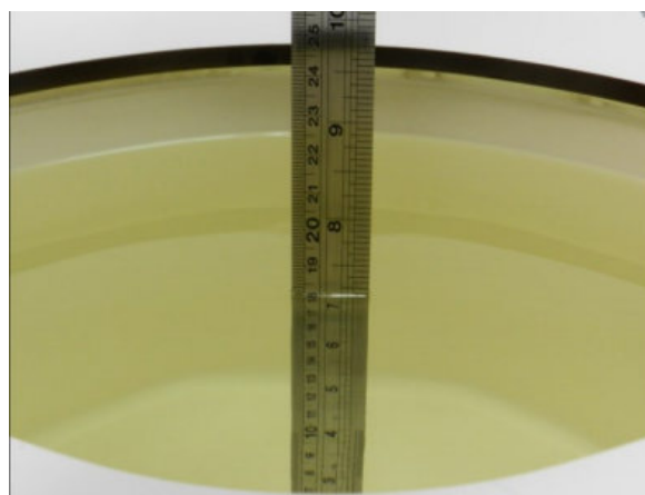
Fig 10.2 Photo of Liquid Height for Body SAR
