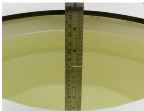
Fig 10.2 Photo of Liquid Height for Body SAR
