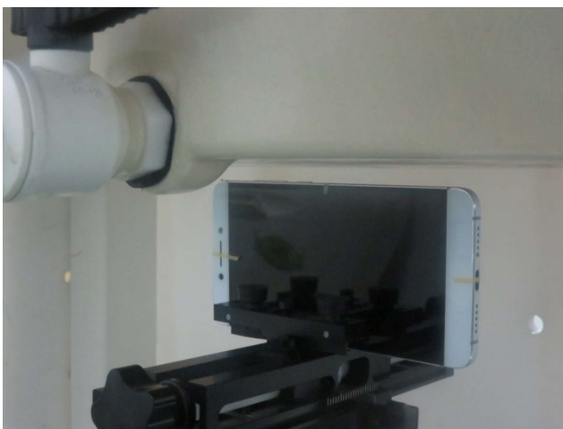
Right Side, Test Separation 10 mm
