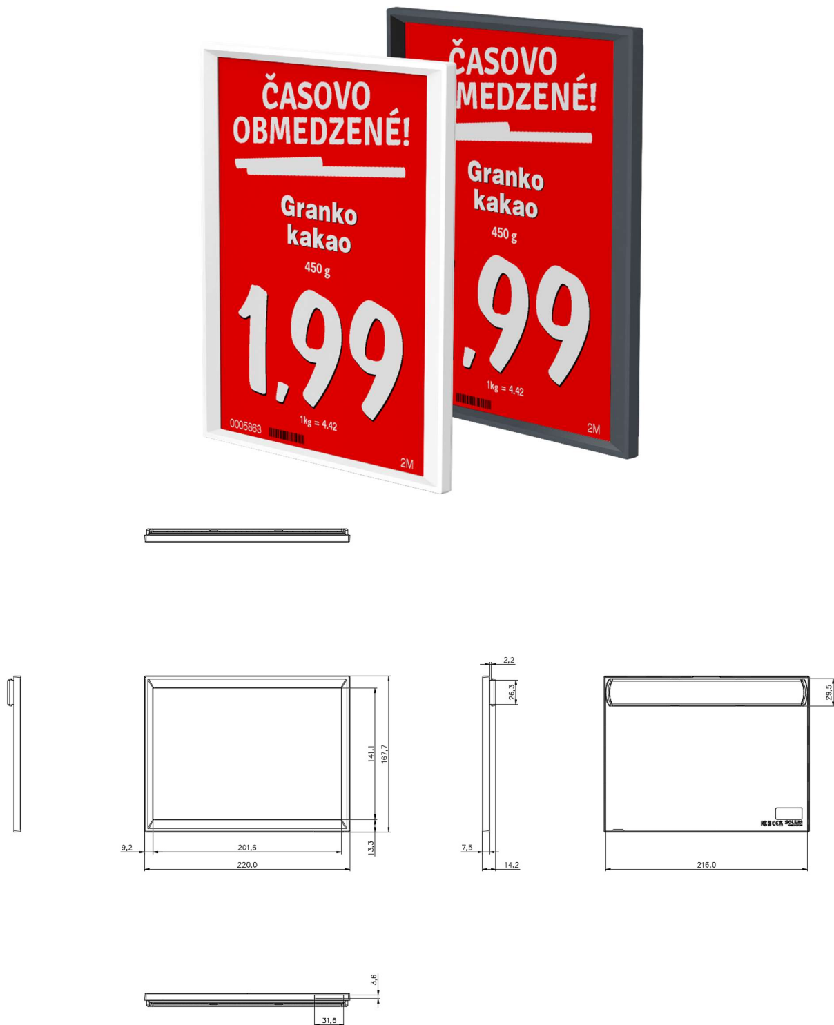
Figure 11. 9.7" 3-COLOR MECHANICAL DIMENSION
