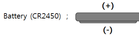
Figure 8. COIN BATTERY DIRECTION
