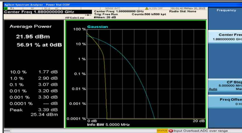
(Channel Bandwidth: 5 MHz)_MCH_QPSK_12RB#13
