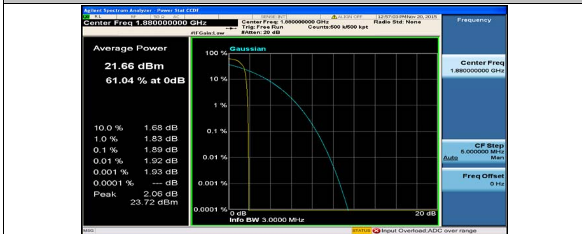
(Channel Bandwidth: 3 MHz)_MCH_16QAM_1RB#7
