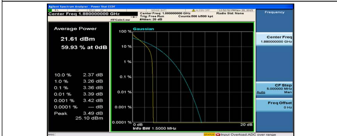
(Channel Bandwidth: 1.4 MHz)_MCH_16QAM_1RB#5
