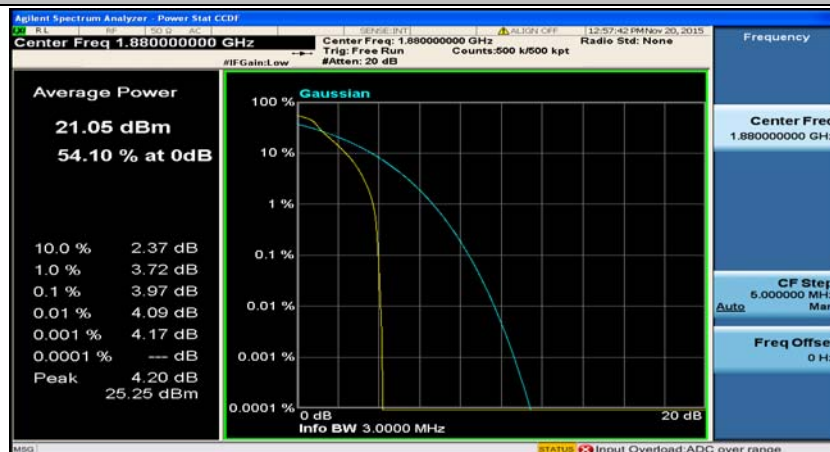
(Channel Bandwidth: 3 MHz)_MCH_16QAM_8RB#7
