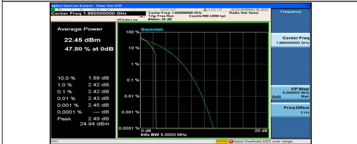
(Channel Bandwidth: 5 MHz)_MCH_QPSK_1RB#24
