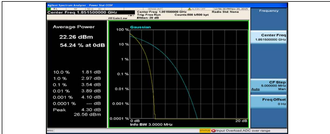
(Channel Bandwidth: 3 MHz)_MCH_QPSK_1RB#0
