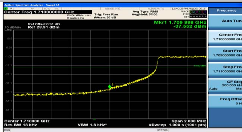
Channel Bandwidth: 10 MHz_LCH_16QAM_25RB#0
