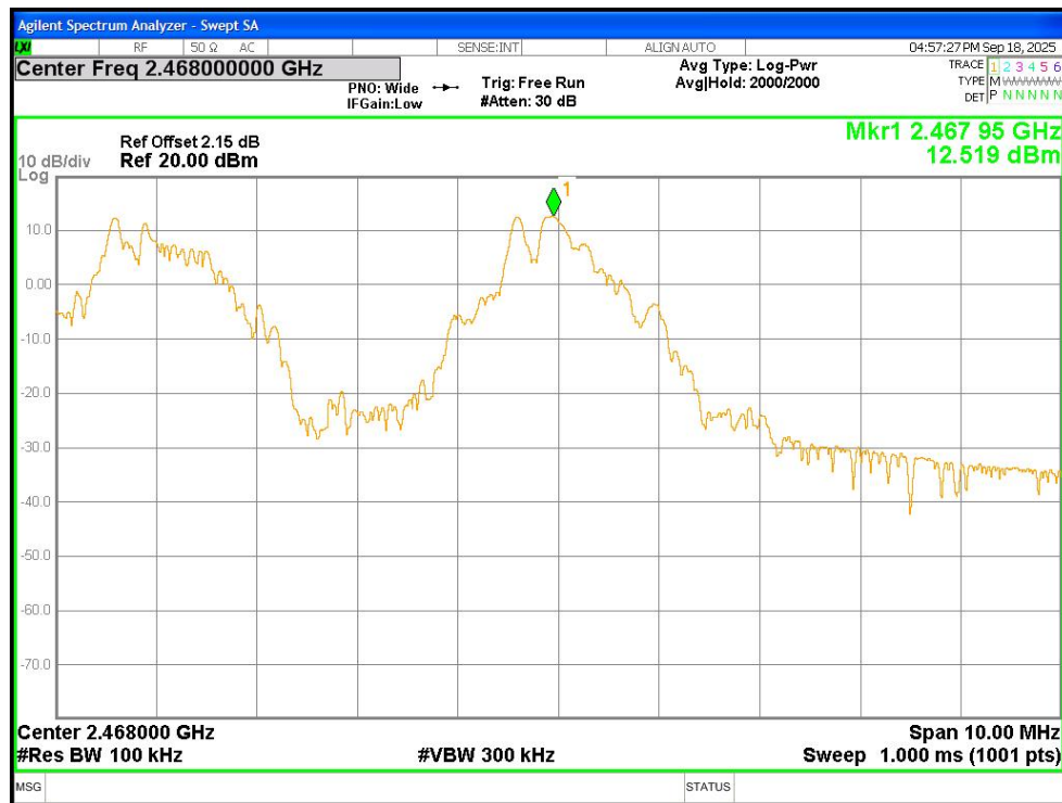
Band Edge(Hopping) NVNT 1-DH1 2468MHz Ant1 Hopping Emission
