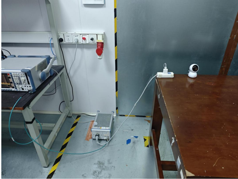
Conducted emissions at AC power line (150kHz-30MHz)
